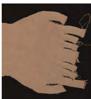
FIGURE 40 Flat knit handpiece before sewing Garments are shaped by adding and removing needles during knitting.
